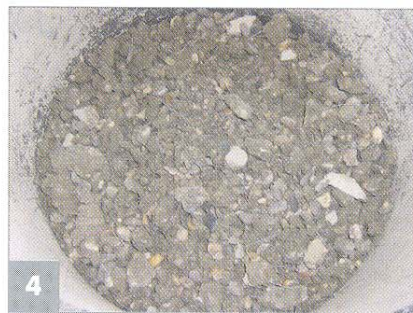
Fibre content determination by crushing hardened concrete test pieces
